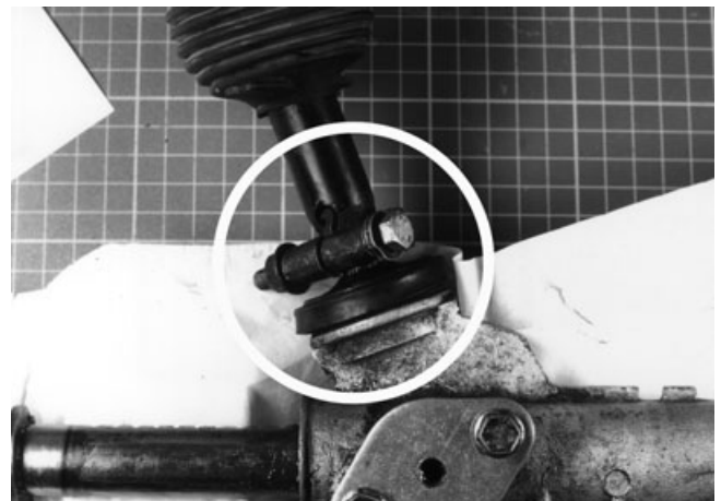
FIG. 4—Photograph of the steering system assembly (upper view). The wheel system is assembled properly, with the bolt screwed all the way.
